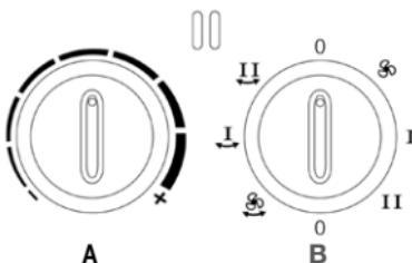
Connect the power supply, indicator light is lit, rotate the switch knob (B). Move the knob (A) to adjust the heating temperature.
