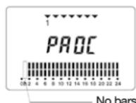
Programming is performed hour by hour. The selected hour will flash.
