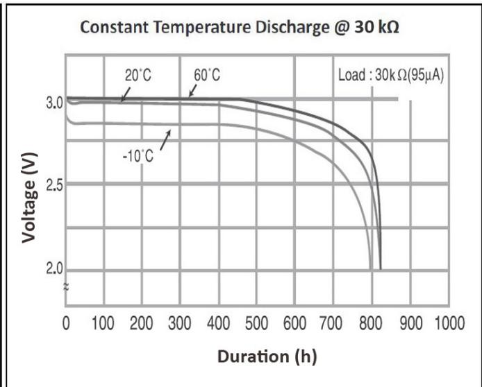
\* Nominal capacity indicates duration until the voltage drops down to 2.0V when discharged at a nominal discharge current at 20°C.
